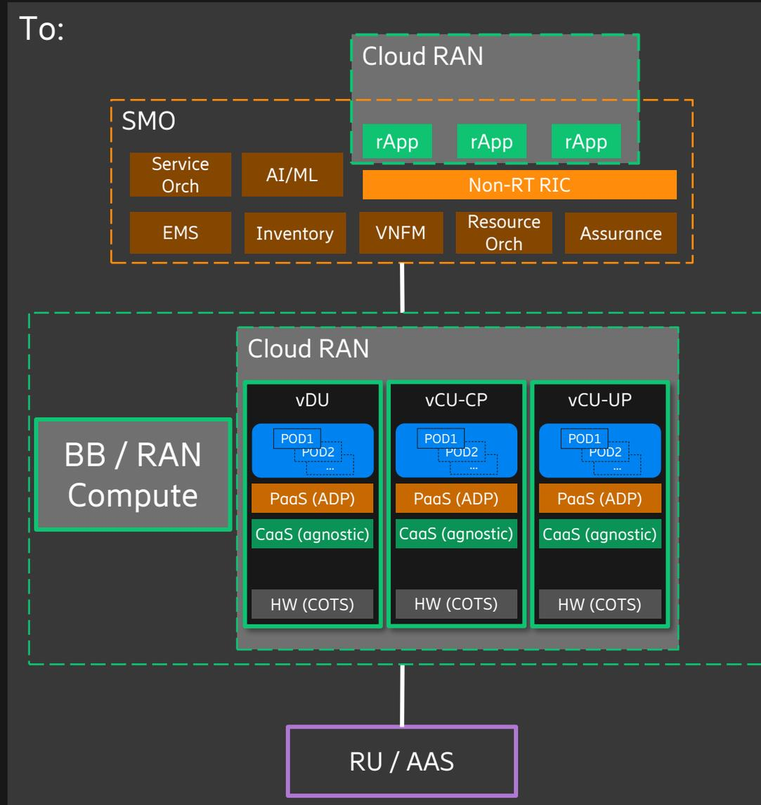
Disaggregation of RAN: vDU, vCU-CP, vCU-UP, rApps.
