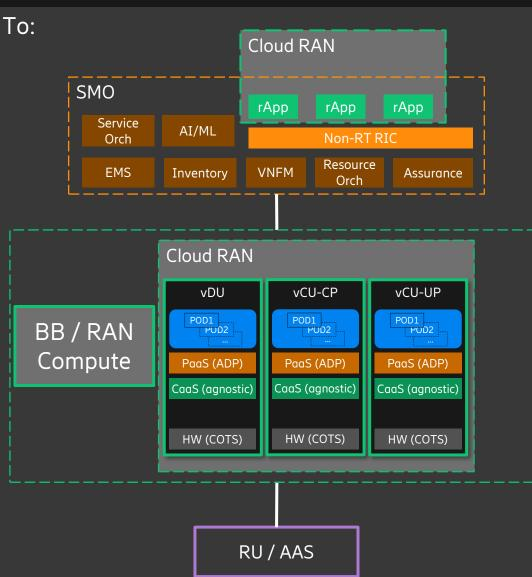
Disaggregation of RAN: vDU, vCU-CP, vCU-UP, rApps.
